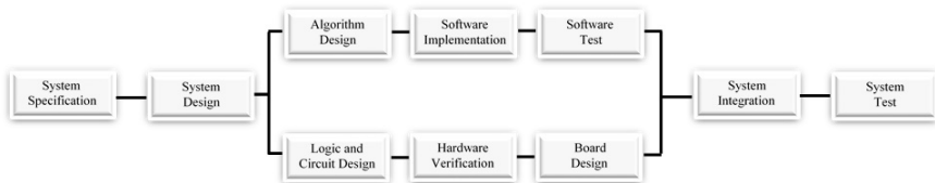
FIGURE – Typical Embedded System Software and Hardware Design Flow
